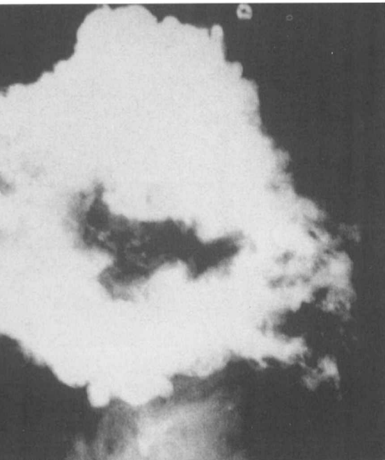
(a) Laboratory simulation of buoyant fluid inside a thermal. After advancing 1 to 2 diameters, a mass of buoyant fluid has formed. Environmental fluid entrained into its core produces a hole in the center of the buoyant mass. (b) Motion and streamlines of a buoyant fluid mass. Mixing with surrounding fluid causes the advancing mass to expand at an angle from the vertical of about 12° to 15° (Kroger (1978)).
