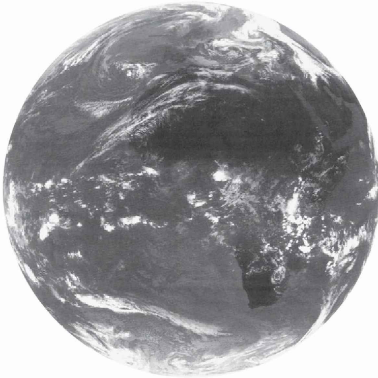
Figure 1.28 Infrared image at 1200 UT on March 4, 1984, from the 11\text{-}\mu\text{m} channel of Meteosat-2. Gray scale displays equivalent blackbody temperature from warmest (black) to coldest (white). (See Fig. 1.29 for geographical landmarks). Supplied by the European Space Agency.
