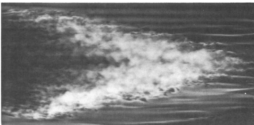
Figure 13.2 Turbulent spot introduced into a laminar flow (from right to left) at Re = 4.0 \cdot 10^5 . After Van Dyke (1982).
